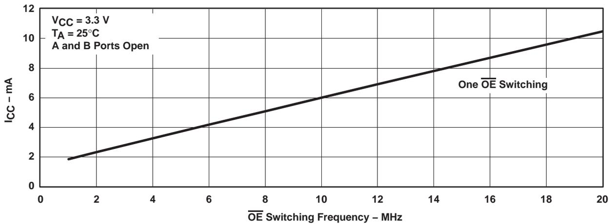
Figure 2. Typical I<sub>CC</sub> vs OE Switching Frequency
